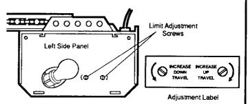
The following chart outlines adjustment procedures. Run the opener through a COMPLETE TRAVEL CYCLE AFTER EACH ADJUSTMENT. NOTE: REPEATED OPERATION OF THE OPENER DURING ADJUSTMENT PROCEDURES MAY CAUSE MOTOR TO OVERHEAT AND SHUT OFF. SIMPLY WAIT 15 MINUTES AND TRY AGAIN. Read chart carefully before proceeding to Step 2. Use a screwdriver to make limit adjustments.
